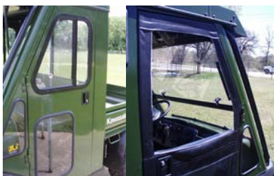
Lightweight Fabric covered doors fit all cabs. They feature a large zippered top window
