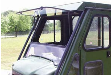
Unique, Glass Lift Windshield and Lift-off front hinged Steel or Fabric doors.
