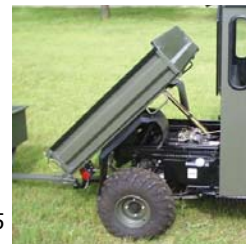
2530EBL: Fast acting Electric Bed Lift is half the cost of a hydraulic lift and works just as well.
