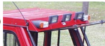
Halogen Lights: Visor and roof mounted Light bars feature 3 to 5 spot and trapezoid Halogen lamps. Bed and Side light kits come with harness and switches. May Require battery and possibly alternator upgrades.
