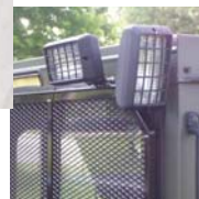
Halogen Lights: Visor and roof mounted Light bars feature 3 to 5 spot and trapezoid Halogen lamps. Bed and Side light kits come with harness and switches. May Require battery and possibly alternator upgrades.
